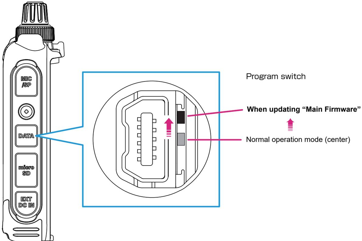
4. Use the supplied USB cable to connect the FT5DR/DE DATA jack to the computer.
