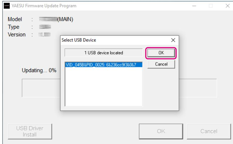
The firmware transfer starts and the FT5DR/DE firmware update executes (it takes about Main Firmware: 20 seconds or Sub Firmware: 90 seconds to complete the update). When the firmware update completes, a message appears.
