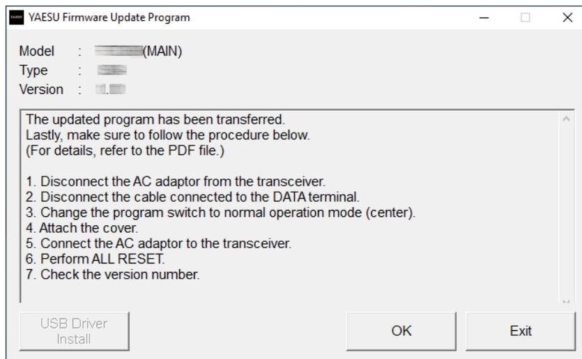
12. Disconnect the AC adaptor from the transceiver.
